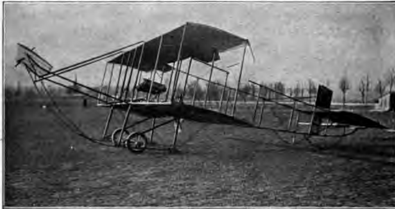
Fig. 24. Sommer Biplane Equipped with Gnome Seven-Cylinder Motor
